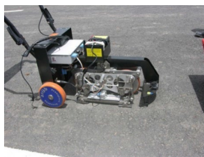
Figure 10. Walking Profiler for measuring road surface profiles
